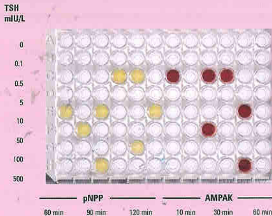
A direct comparison between AMPAK and pNPP in a quantitative TSH assay
